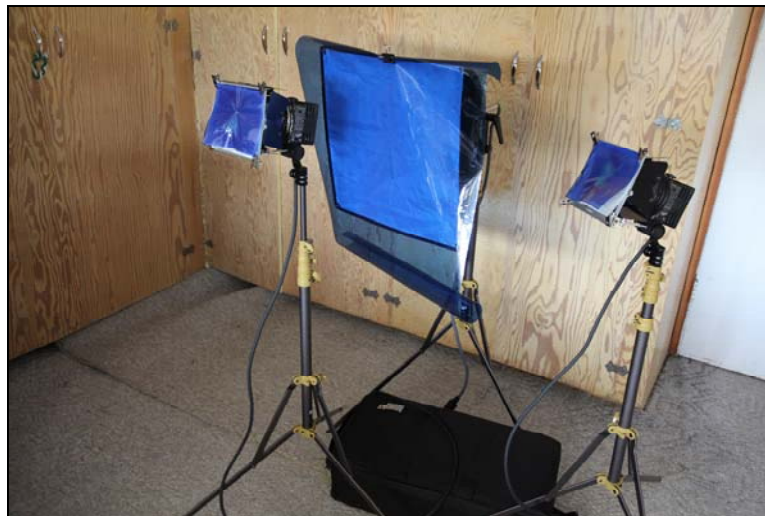
Figure 4-9: Blue gels balance incandescent light with daylight.
